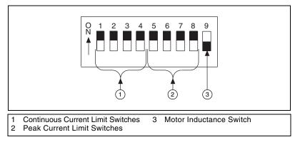
Figure 3. 9-Position DIP Switch Bank Layout
